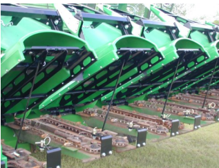
30" Bifold 843JD hinged on rear for maintenance.
