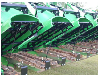
30" Bifold 843JD hinged on rear for maintenance.
